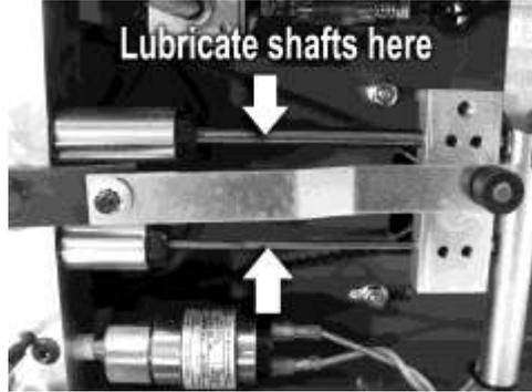
To lubricate both air pistons **ONLY USE WHITE LITHIUM GREASE**. Disassembly of the pistons is not required. Simply put a dab of grease on the exposed piston shaft near the end of the cylinder. Once the unit is turned on, the grease will get pulled into the cylinder as the piston moves in and out. See our website videos on the Support page at [Shoeboxcompressor.com](http://Shoeboxcompressor.com)
